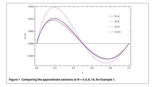
approximate solutions at  $\alpha = \beta = -\frac{1}{2}$  and a few collocation points (N = 4, 6, 8, 16) of this problem are depicted in Figure 1. The approximate solution at N = 8 agrees very well with the approximate solution at N = 16; this means the numerical solution converges fast as N increases.
