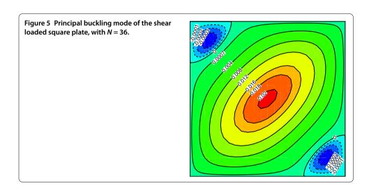
Example 3 (Shear loaded square plate) In this example, we chose the plane stress field
