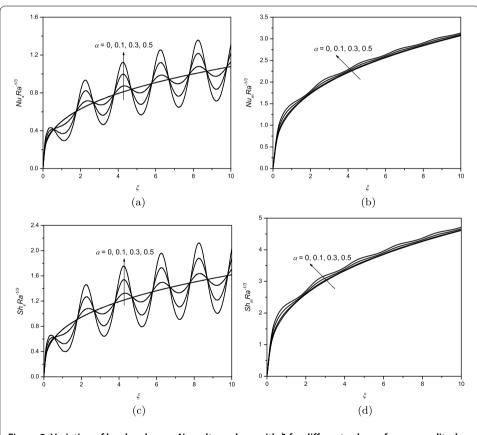
Figure 5 Variation of local and mean Nusselt numbers with  $\xi$  for different values of wave amplitude  $\alpha$  with N=1, Le=2, and  $D_f=Sr=0$ .
