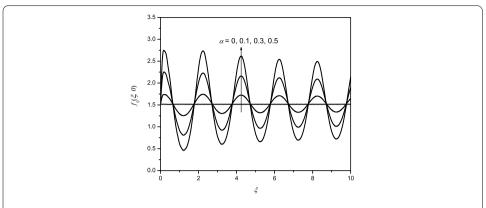
Figure 4 Variation of slip velocity  $f_{\eta}(\xi,0)$  with  $\xi$  for varying wave amplitude  $\alpha$  with N=1, Le=2, and  $D_f=Sr=0$ .
