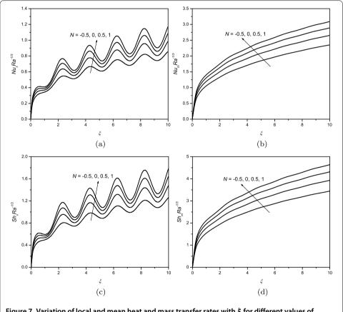
Figure 7 Variation of local and mean heat and mass transfer rates with  $\xi$  for different values of buoyancy number N with  $\alpha = 0.2$ , Le = 2, and  $D_f = Sr = 0$ .
