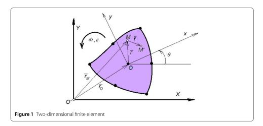
current point with the coordinates expressed in the mobile system,  $\{\delta\}_L$  is the vector of nodal coordinates, [N] is the shape function matrix, [R] represents the rotation matrix that makes the transition from the mobile reference system to the fixed reference system, and  $[\dot{R}]$  is the derivative of [R] with respect to time.
