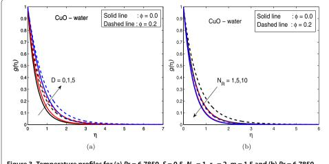
Figure 3 Temperature profiles for (a) Pr = 6.7850, S = 0.5,  $N_R = 1$ ,  $r_1 = 2$ , m = 1.5 and (b) Pr = 6.7850, S = 0.5, D = 1,  $r_1 = 2$ , m = 1.5.
