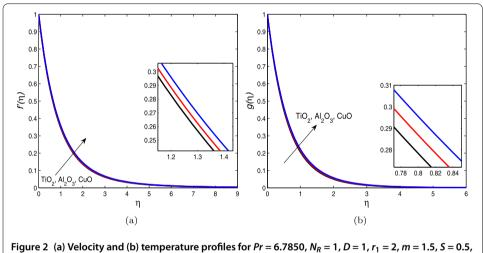
Figure 2 (a) Velocity and (b) temperature profiles for Pr=6.7850,  $N_R=1$ , D=1,  $r_1=2$ , m=1.5, S=0.5,  $\phi=0.2$ .
