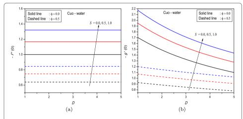
Figure 6 (a) Skin friction and (b) heat transfer coefficients as a function of D, when Pr = 6.7850,  $N_R = 1$ ,  $r_1 = 2$ , m = 1.5.
