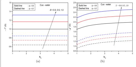
Figure 5 (a) Skin friction and (b) heat transfer coefficients as a function of  $N_R$ , when Pr = 6.7850, D = 1,  $r_1 = 2$ , m = 1.5.
