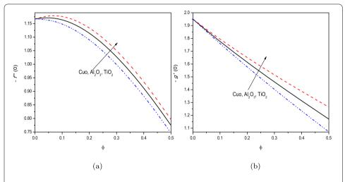
Figure 4 (a) Skin friction and (b) heat transfer coefficients as a function of nanoparticle volume fraction, when Pr = 6.7850, S = 0.5, D = 1,  $N_R = 1$ ,  $r_1 = 2$ , m = 1.5.
