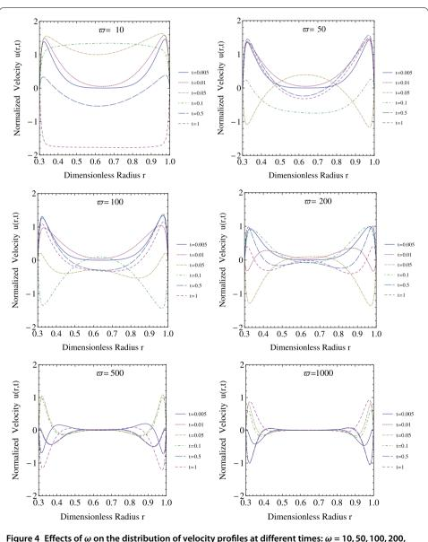
Figure 4 Effects of  $\omega$  on the distribution of velocity profiles at different times:  $\omega$  = 10, 50, 100, 200, 500, 1,000.
