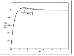
Figure 4 The influence of the chemical reaction parameter on the horizontal velocity for with  $\lambda=0.5; R=1; Pr=0.71; \lambda_1=0.5; \lambda_2=0.5;$   $Ec=0.1; \delta=0.1; M=0.5; \delta=0.1; Sc=0.22.$
