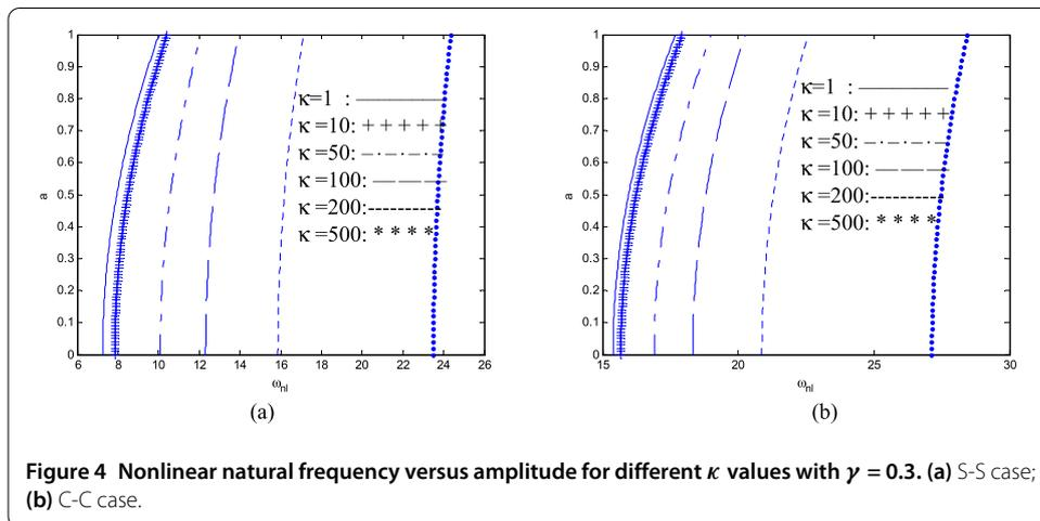
**Figure 4** Nonlinear natural frequency versus amplitude for different  $\kappa$  values with  $\gamma = 0.3$ . (a) S-S case; (b) C-C case.
