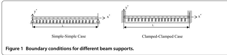
**Figure 1** Boundary conditions for different beam supports.
