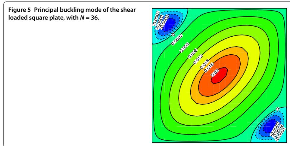
**Example 3** (Shear loaded square plate) In this example, we chose the plane stress field
