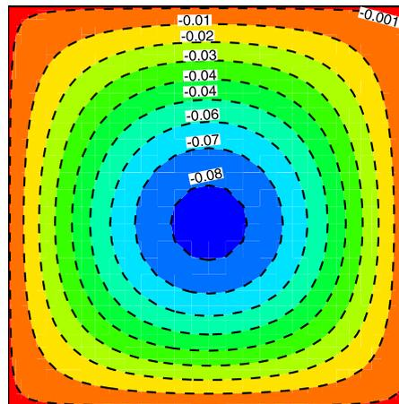
**Figure 4** Principal buckling mode corresponding to  $\alpha = 1$ , with  $N = 36$ .
