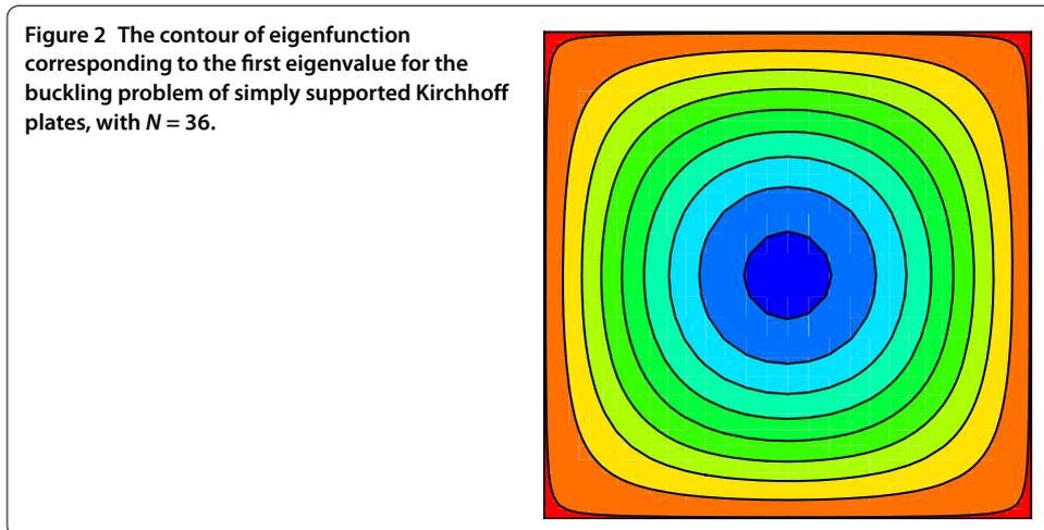
Kirchhoff plates. These results demonstrate that our approach can achieve an exponential convergence rate which is in good agreement with the theoretical result. Moreover, Figure 2 shows the contour line of eigenfunction corresponding to the lowest buckling coefficient of the buckling problem.
