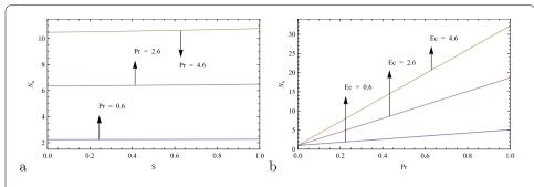
**Figure 13** (a) The effect of Nusselt number for different values of Pr. (b) The effect of Nusselt number for different values of Ec. With fixed values are Sc = 1.5, Bt = 0.3,  $\delta = 1.0$ ,  $\alpha_1 = 1.2$ ,  $\alpha_2 = 1.8$ , B = 1.7, S = -1.1,  $K_1 = 1.8$ ,  $K_2 = 2.6$ ,  $\Omega = 1.2$ ,  $\lambda = 0.3$ , Ec = 0.3, Ec = 0.3,
