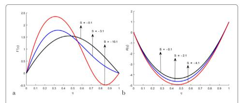
**Figure 2** Profile of  $f'(\eta)$  and  $\theta(\eta)$  for different values of *S* and fixed values of Sc = 1.5,  $\delta = 1.0$ ,  $\alpha_1 = 1.2$ ,  $\alpha_2 = 1.8$ , Bt = 0.3, B = 1.7,  $K_1 = 1.8$ ,  $K_2 = 0.6$ , Pr = 1.6, Ec = 0.5
