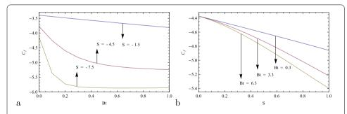
**Figure 12** (a) The effect of skin friction for different values of *S*. (b) The effect of skin friction for different values of *Bt*. With fixed values are Sc = 1.5, Bt = 0.3,  $\delta = 1.0$ ,  $\alpha_1 = 1.2$ ,  $\alpha_2 = 1.8$ , B = 1.7, S = -1.1,  $K_1 = 1.8$ ,  $K_2 = 2.6$ ,  $\Omega = 1.2$ ,  $\lambda = 0.3$ , Ec = 0.3, Ec
