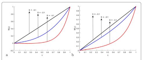
**Figure 3** Profile of  $N(\eta)$  and  $M(\eta)$  for different values of S and fixed values of Sc = 1.5,  $\delta = 2.0$ ,  $\alpha_1 = 1.2$ ,  $\alpha_2 = 0.4$ , Bt = 0.3, B = 1.7,  $K_1 = 1.8$ ,  $K_2 = 2.6$ , Pr = 0.6, Ec = 3.5
