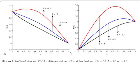
**Figure 4** Profile of  $H(\eta)$  and  $K(\eta)$  for different values of *S* and fixed values of Sc = 0.5,  $\delta = 2.0$ ,  $\alpha_1 = 1.2$ ,  $\alpha_2 = 0.4$ , Bt = 0.3, B = 1.7,  $K_1 = 1.8$ ,  $K_2 = 2.6$ , Pr = 0.6, Ec = 3.5
