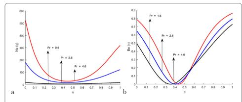
**Figure 9** Profile of  $N_s(η)$  and  $B_e(η)$  for different values of  $P_r$ ,  $E_c$  and fixed values of  $S_c = 1.5$ ,  $B_t = 0.3$ ,  $\delta = 4.0$ ,  $\alpha_1 = 1.2$ ,  $\alpha_2 = 1.8$ , B = 1.7, S = -1.1,  $K_1 = 1.8$ ,  $K_2 = 2.6$ ,  $\Omega = 1.2$ ,  $\lambda = 0.3$ ,  $E_c = 0.5$
