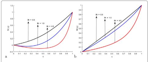
**Figure 5** Profile of  $N(\eta)$  and  $M(\eta)$  for different values of  $B_t$  and fixed values of Sc = 1.5,  $\delta = 4.0$ ,  $\alpha_1 = 1.2$ ,  $\alpha_2 = 1.8$ , B = 1.7, S = -1.1,  $K_1 = 1.8$ ,  $K_2 = 2.6$ , Pr = 1.6, Ec = 0.5
