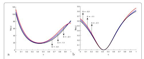
**Figure 8** Profile of  $N_s(\eta)$  and  $B_e(\eta)$  for different values of S and fixed values of Sc = 0.5,  $\delta$  = 2.0,  $\alpha_1$  = 1.2,  $\alpha_2$  = 0.4, Bt = 0.3, B = 1.7,  $K_1$  = 1.8,  $K_2$  = 2.6, Pr = 1.6, Ec = 0.5,  $\Omega$  = 1.2,  $\lambda$  = 0.3
