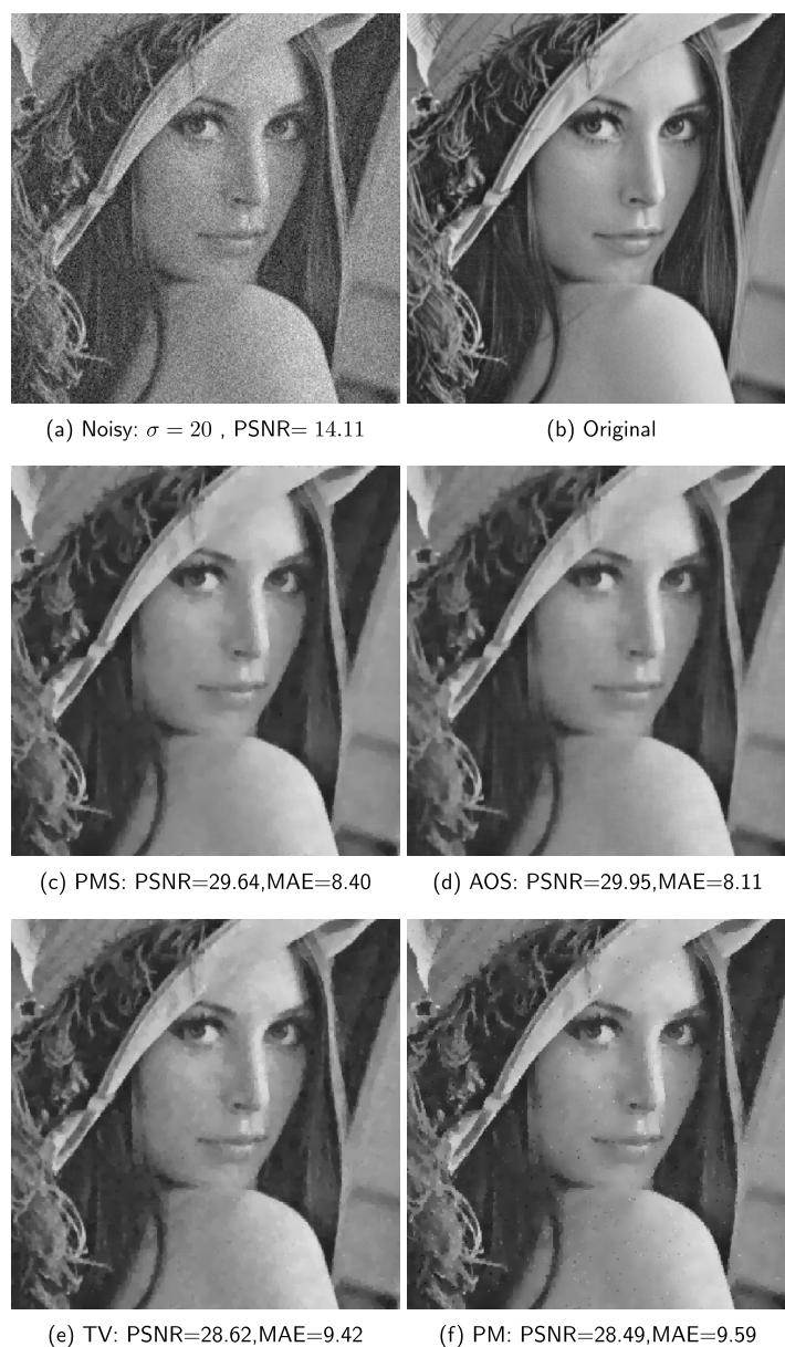
Figure 4 Lena image ( 300 \times 300 ): (a) noisy image corrupted by Gaussian noise for \sigma = 20 ; (b) original image; (c) our algorithm by PMS, \mu_1 = 0.3 , \mu_2 = 0.7 , and \tau = 0.2 ; (d) our algorithm by AOS, \mu_1 = 0.9 , \mu_2 = 0.1 , and \tau = 2 ; (e) TV algorithm, \tau = 0.2 ; and (f) PM algorithm, \tau = 0.2 and K = 5
