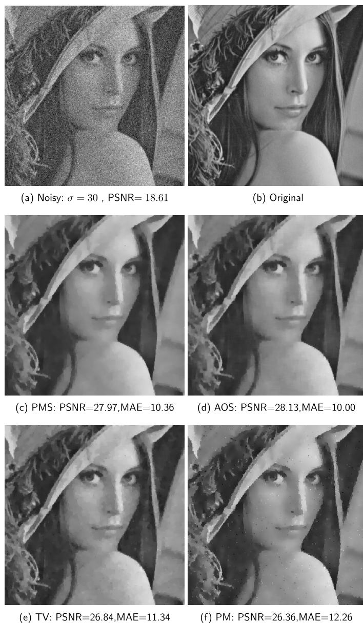
Figure 5 Lena image ( 300 \times 300 ): (a) noisy image corrupted by Gaussian noise for \sigma = 30 ; (b) original image; (c) our algorithm by PMS, \mu_1 = 0.5 , \mu_2 = 0.5 , and \tau = 0.2 ; (d) our algorithm by AOS, \mu_1 = 0.9 , \mu_2 = 0.1 , and \tau = 2 ; (e) TV algorithm, \tau = 0.2 ; and (f) PM algorithm, \tau = 0.2 and K = 7
